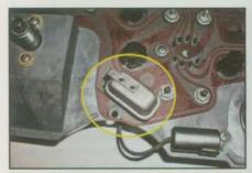
The factory calls the 5-volt instrument regulator a "limiter" (it's not). But it does supply the reference voltage for the gauges. The most common style is the PCB plug-in one shown here. Some cars, notably those with no PCB, use a different case and terminals, some have it built into a gauge. In all cases the function is identical.
