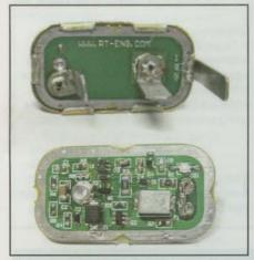
We devised a cheap solid-state replacement for the stock electromechanical regulator a decade ago, but the latest one from Real Time Engineering (bottom) is much better. (Photo: G. Garner)
