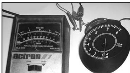
10. Now check the calibration at two points: 1000 and 4000 RPM. Turn the small screws to make your tach agree with the reference tach—try to use a good digital tune-up tach, not our cheapo swap-meet analog junk! (In other words, do as we say, not as we do!) Now just bolt it all back together—done!
